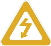
The LIGHTNING flash symbol is intended to alert you to the presence of uninsulated "dangerous voltage" within the product's enclosure that may be sufficient magnitude to constitute a risk of electrical shock.
